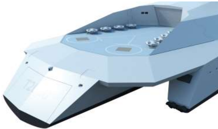
Above, tethered quadcopter mast; below, UAV aviation deck; bottom, UUV 'garage'
