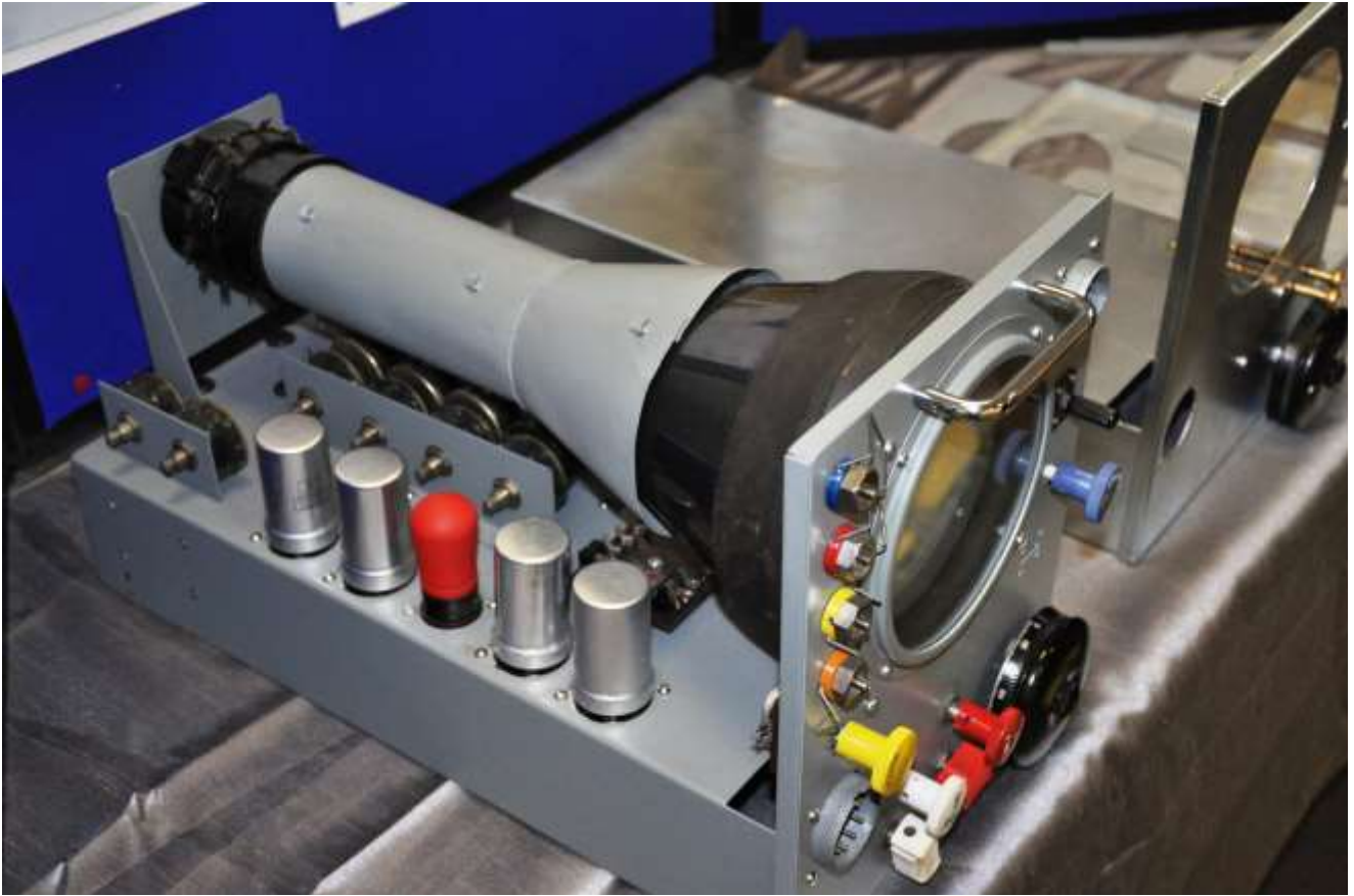
GEE Mk I Indicator under construction, showing ERT's immaculate detailing of metalwork and their close attention to detail
