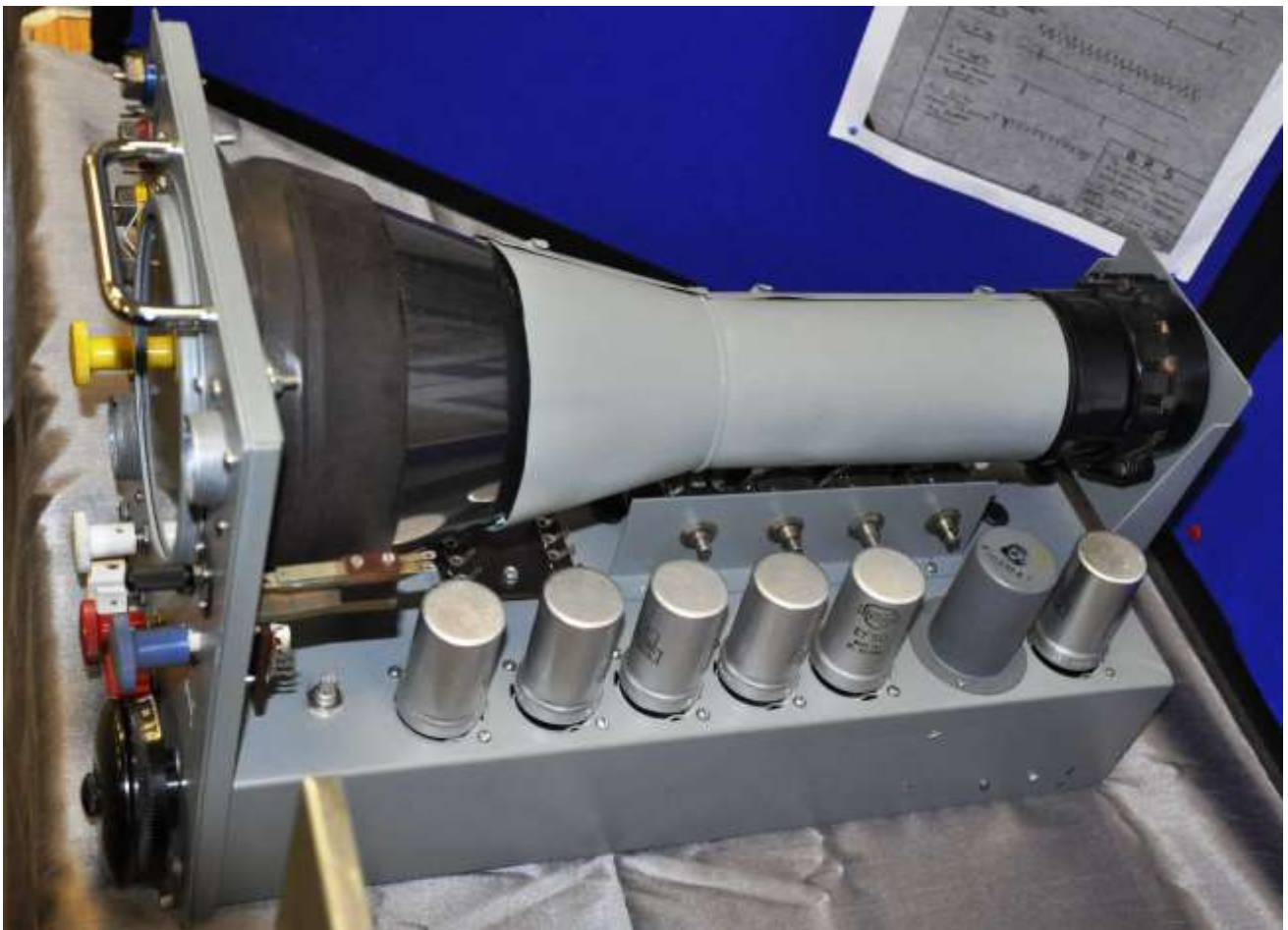
GEE Mk I Indicator under construction, showing ERT's immaculate detailing of metalwork and their close attention to detail
