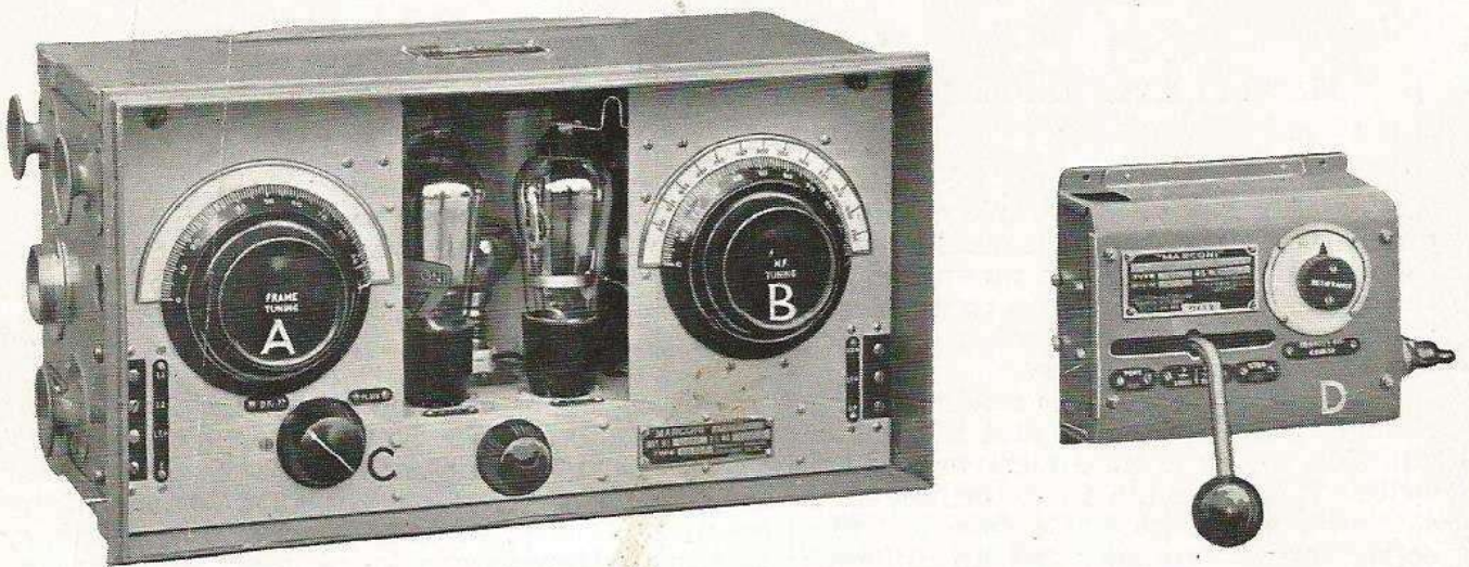
MARCONI TYPE AD 52 AMPLIFYING ATTACHMENT AND LOOP REVERSING SWITCH FOR MARCONI AIRCRAFT D.F. EQUIPMENT.
