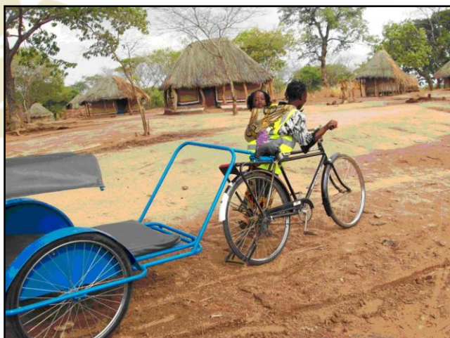
Figure 4. The "Namibian" style of bicycle ambulance constructed during the Zambia project.
