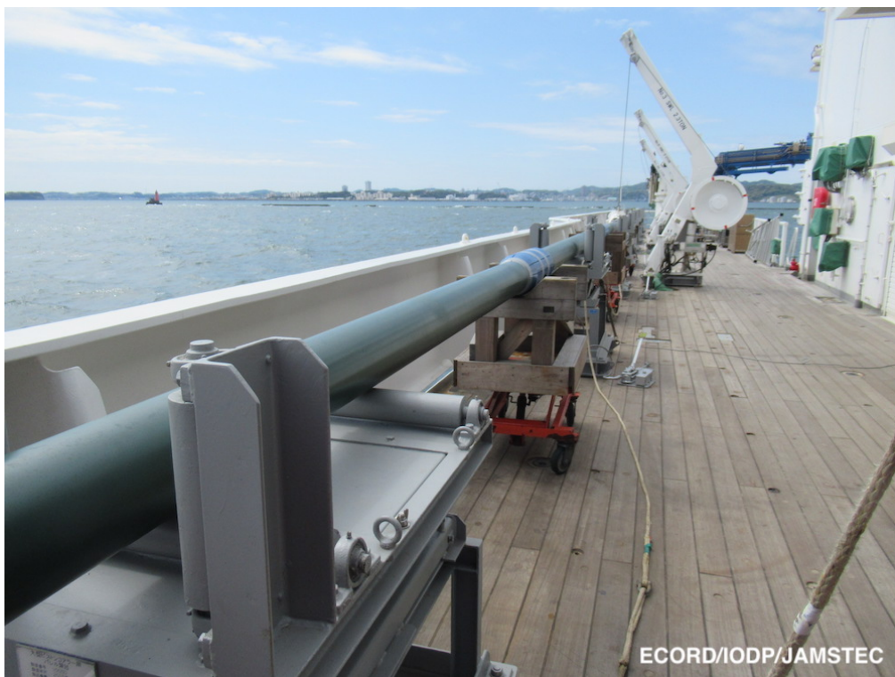
20 m Giant Piston Corer ready to go (photo by NSakurai@ECORD/IODP/JAMSTEC)
