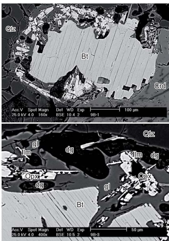
FIG. 3-16. a) Backscattered SEM image of a microstructure such as in Fig 3-15a. Note the kinetic control on reaction progress, with extensive reaction at the boundaries with quartz, and little or no reaction at the boundaries with cordierite. b) Close-up of a reaction rim around biotite, displaying fresh (gl) and weathered (dg) glass, elongate orthopyroxene and acicular to dendritic ilmenite.
