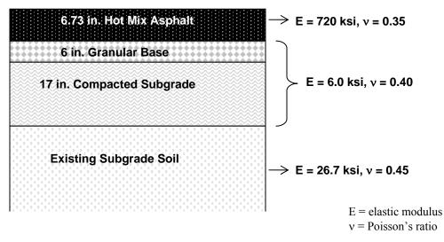
Figure 4. Cross Section of Test Section N5.
