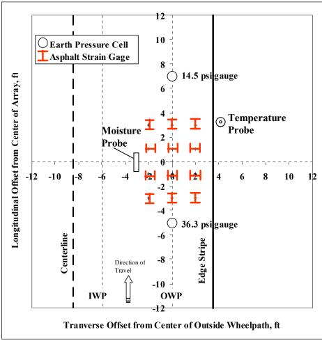
**Figure 9. Instrumentation Schematic.**
