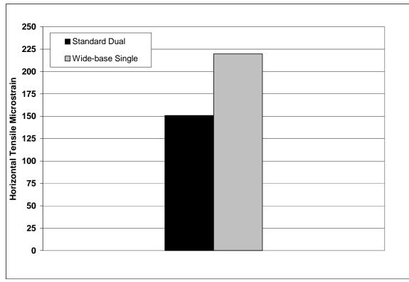
Figure 7. Calculated Horizontal Strain at the Bottom of the Asphalt Layer.
