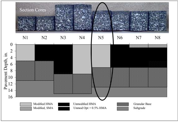
Figure 10. Structural Study Test Section Profile.
