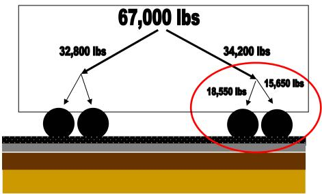
Figure 6. Test Vehicle Weight Distribution.
