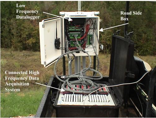
Figure 13. Data Acquisition System.
