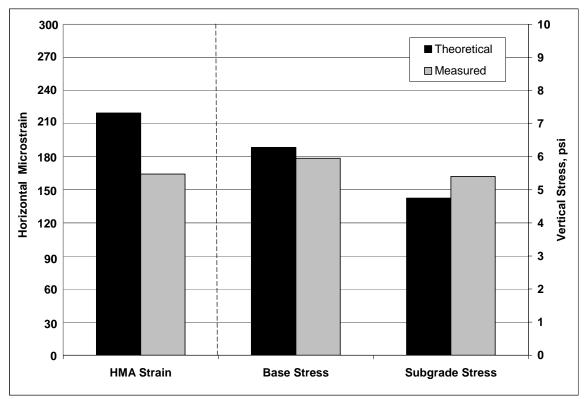
Figure 20. Theoretical vs. Measured Response for Wide-base Single Configuration.
