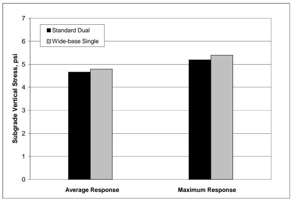
Figure 17. Field Measured Subgrade Stress.
