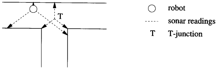
Fig. 12. How the robot NX reaches and recognizes a T-section in a maze. The T-section is characterized by location T, which is defined as the location from where the three sonar readings are equal.
